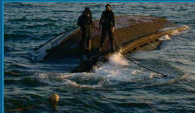
Removal of hydrocarbon from sunken tugboat 'DCI Tug VI', off Nagapattinam, T.N., India.
